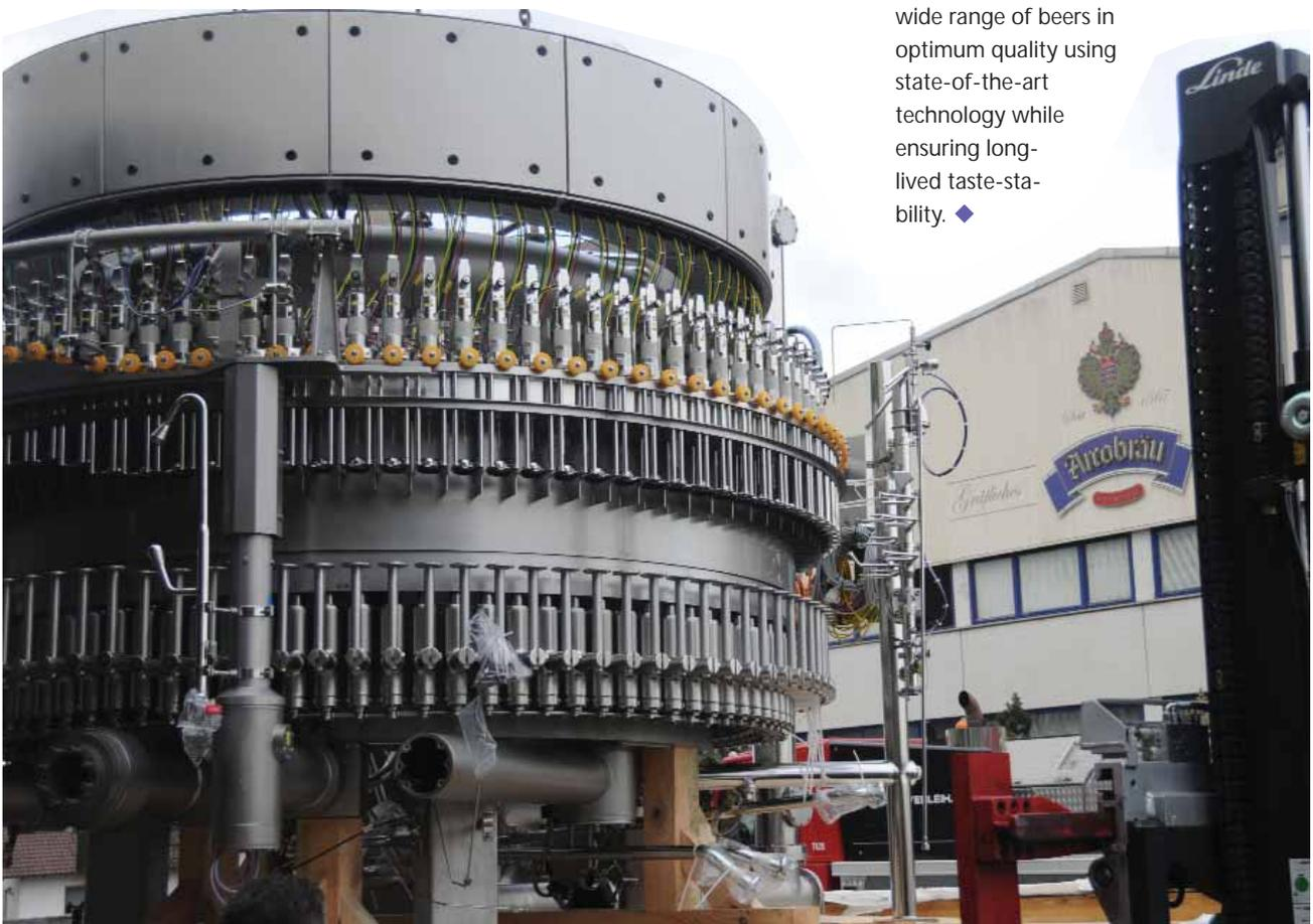
Majestically, the Kronen Modulfill waits to be ingressed at the tradition-steeped Arcobräu Brewery in Moos. Thanks to its low-oxygen-pickup filling process, it will in future ensure maximised taste-stability for Arcobräu's specialty beers.
