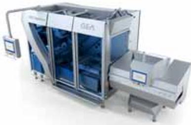
with an extremely large cutting cross-section of 640 x 210 mm. With this it is possible, for example, to slice sausage products six times calibre 105 mm or cheese logs on edge four times 110 x 165 mm
