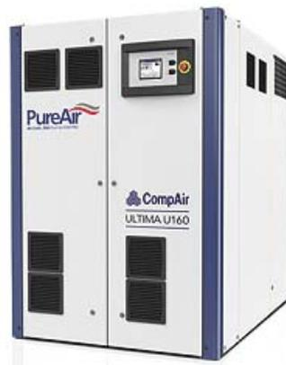
concept - two, high-efficiency, permanent magnet motors which replace the gearbox and single motor. These variable-speed motors, powered by an inverter, can achieve speeds of up to 22,000 rpm and deliver efficiencies greater than IE4.
