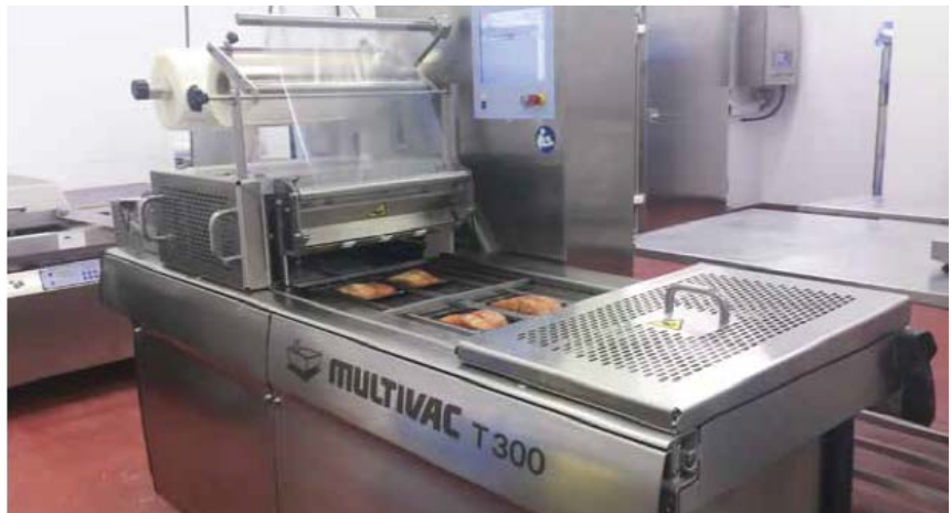
The T 300 is particularly space-saving and is suitable for producing both modified atmosphere packs and vacuum skin packs.
