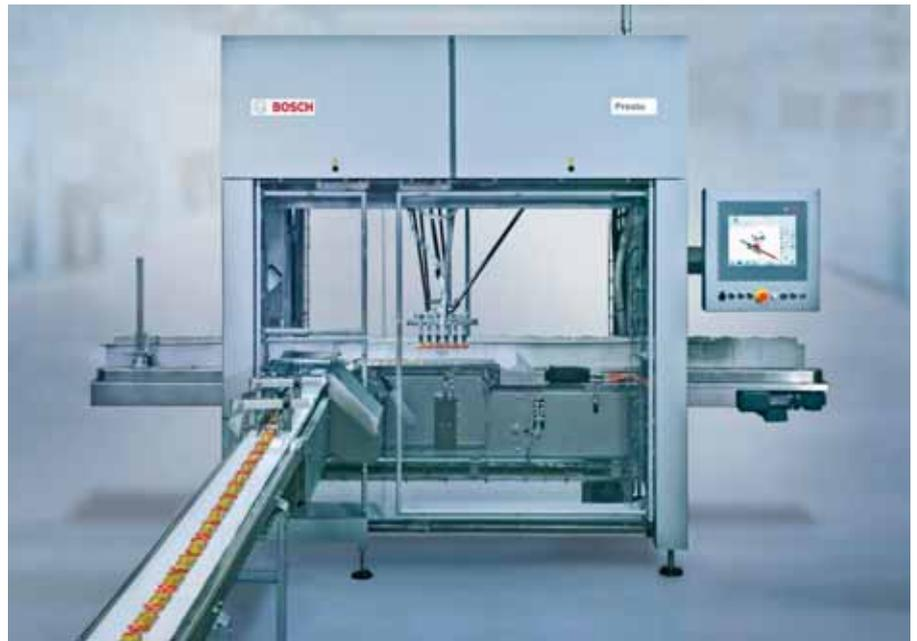
The modular design of Presto D3 toploading collator facilitates handling of multiple product and carton types and sizes on the same machine as per its manufacturer.
