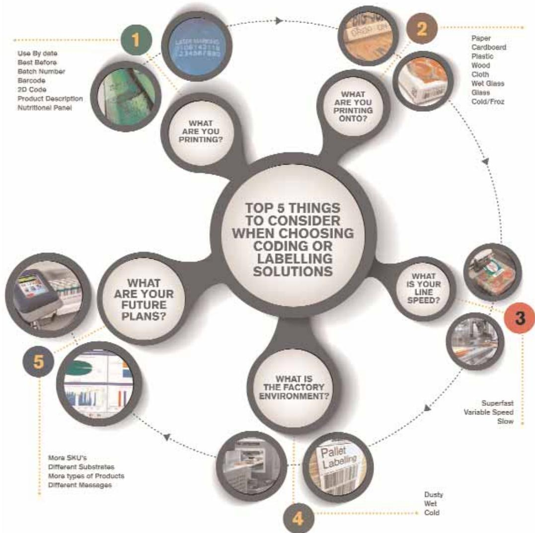
use and storage. Depending on your application, laser coders or continuous inkjet (CIJ) coders or thermal transfer overprinters (TTOs) could be a good choice.
